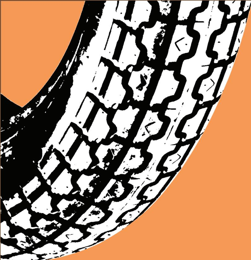
the tire. In the middle the compound is harder and wears longer. On the sides it is softer and gives better traction. Those tires that have grooves all across the tire have wear bars in the middle, and on the side of the tread. It is easy to see the amount of tread left using these wear indicators. Of course the tires with no grooves in the middle leave a lot to be desired.
