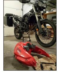
When pulling the tank out, you pull it backwards just enough to get the tank on the higher front perch. This
