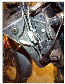
from the grips and switch are strapped to the radiator infill molding and then attached to another wiring harness that runs through the frame and under the tank to the existing bike power plug. At this point everything is hooked up and ready for a test. Don't leave the grips on too long without the motor running as they will run the battery dead.
