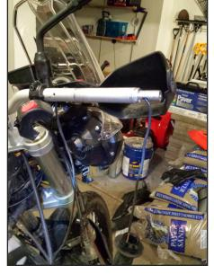
the right hand controls the throttle cables are exposed. Make sure you don't get them mixed up. Next is probably the hardest part of the install. You must thread the heated grip power cable and connectors through a small hole at the end of the handlebars. Once in the handlebars, the cable has to be pushed to another hole near the controls. You then must pull the two connec-
